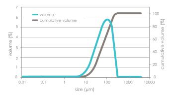
The spherical particle morphology of Plasdone™ \$630 Ultra copovidone improves powder flow characteristics compared with the original copovidone as indicated in Figure 3. Improved powder flow results in a more efficient manufacturing process and minimizes or eliminates feeder clogging and prevents manufacturing stoppages.
